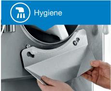
The extraction chute is removable to facilitate the removal of all gelato residue, for complete cleaning.
